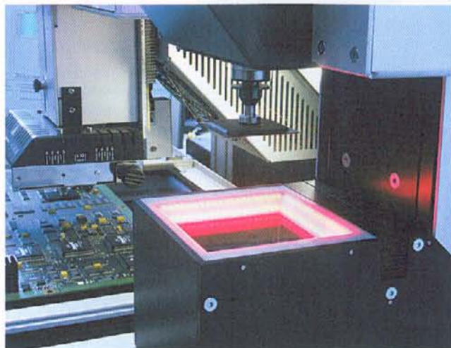
Figure 4: The precision-placement module with auto pick & place function
