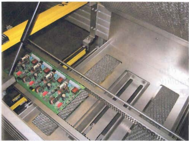
Figure 4: The oven can be equipped with a maximum of two spray heads and separate flux supply
