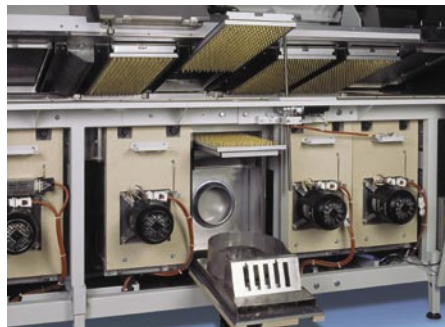
Extracted multijets, opened heater module
