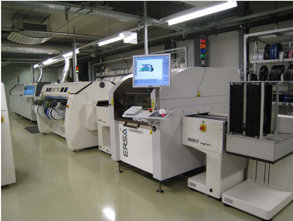
Picture 2: SMT production line with ERSA printer and reflow oven
