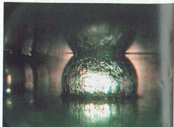
Figure 6. Outer BGA ball with visible upper and lower joints
