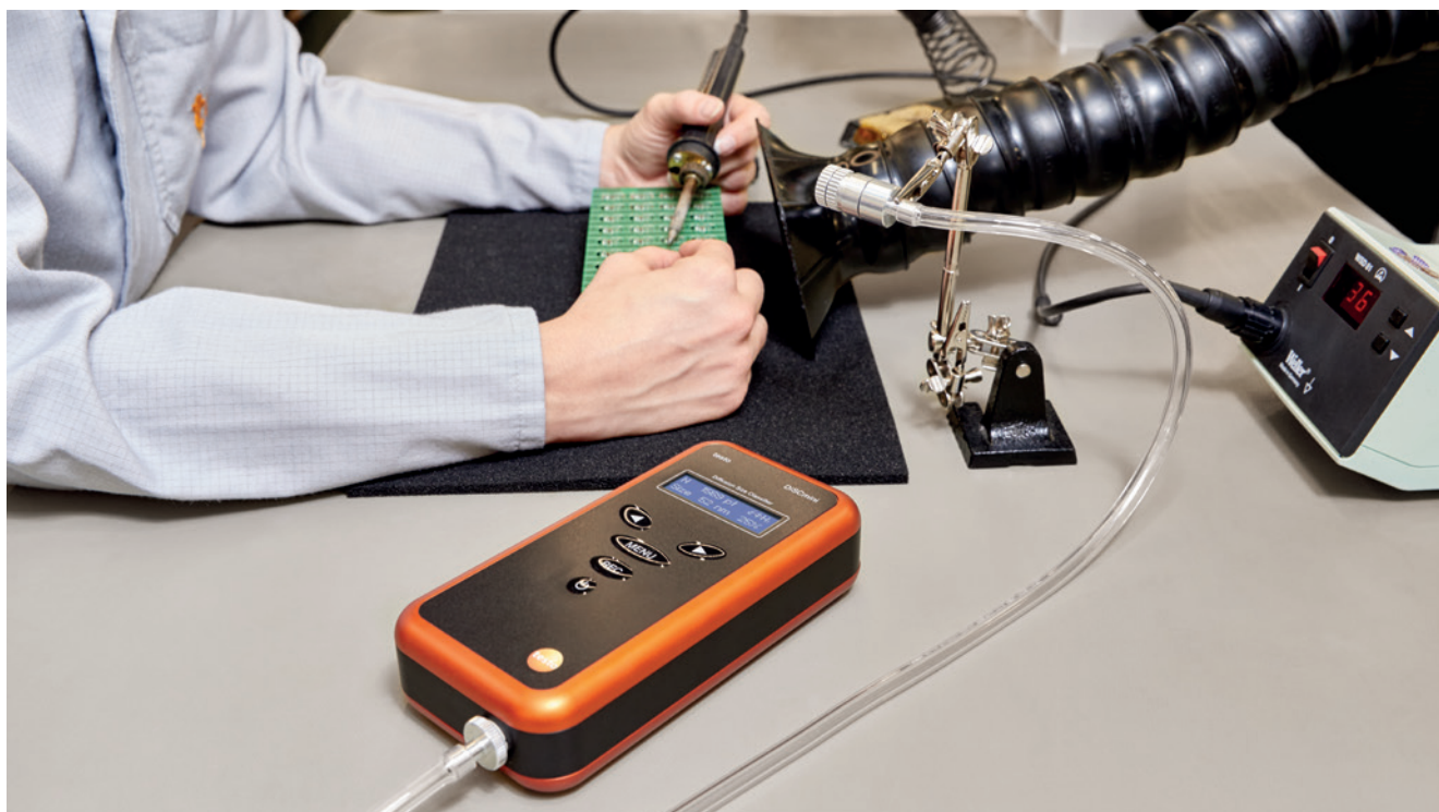
Fig. 2: Setup of the measuring environment with soldering station and extraction.
